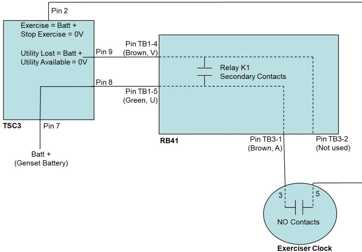
Figure 5 – OPT Transfer Switch RB41 control logic
