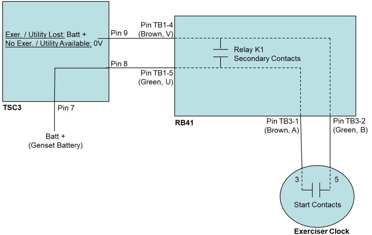
Figure 4 – AST Transfer Switch RB41 control logic
