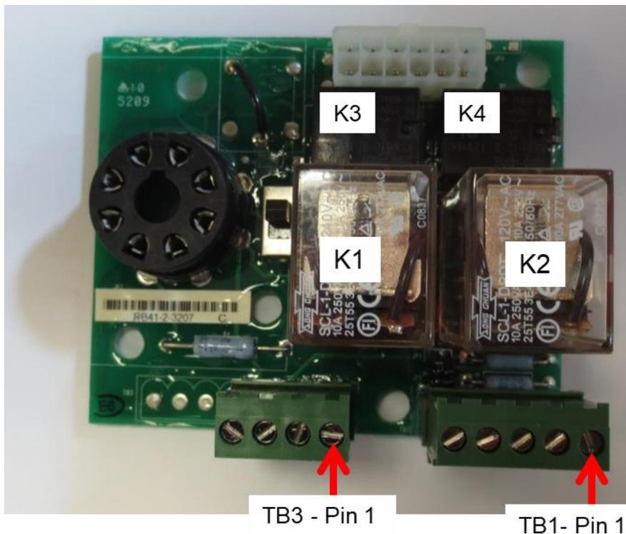
Figure 2 – RB41 Pinout
